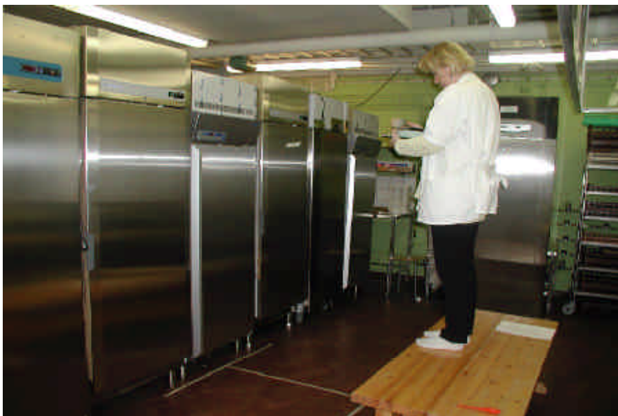
Picture 7. The distance between the appliance and the measuring device was one meter, and the measuring height from the floor was 1,6 meters.
